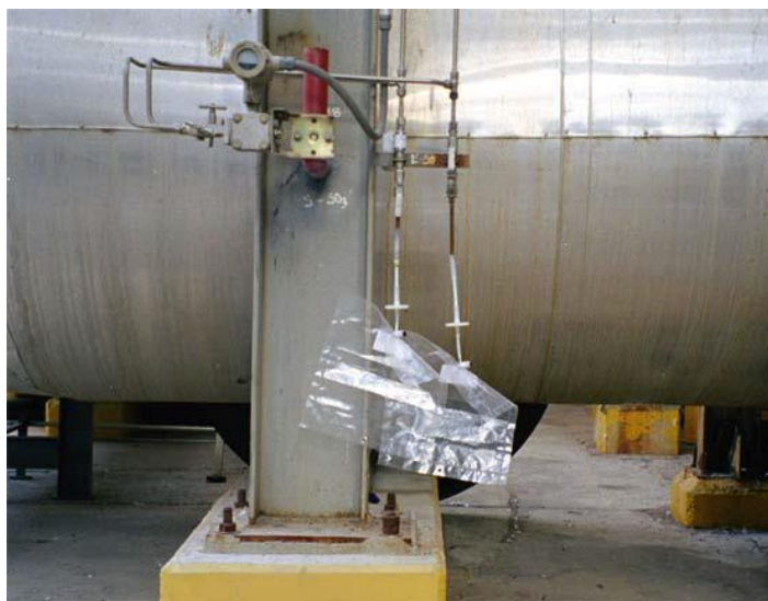
Simultaneously sampling in bags across a heat exchanger
