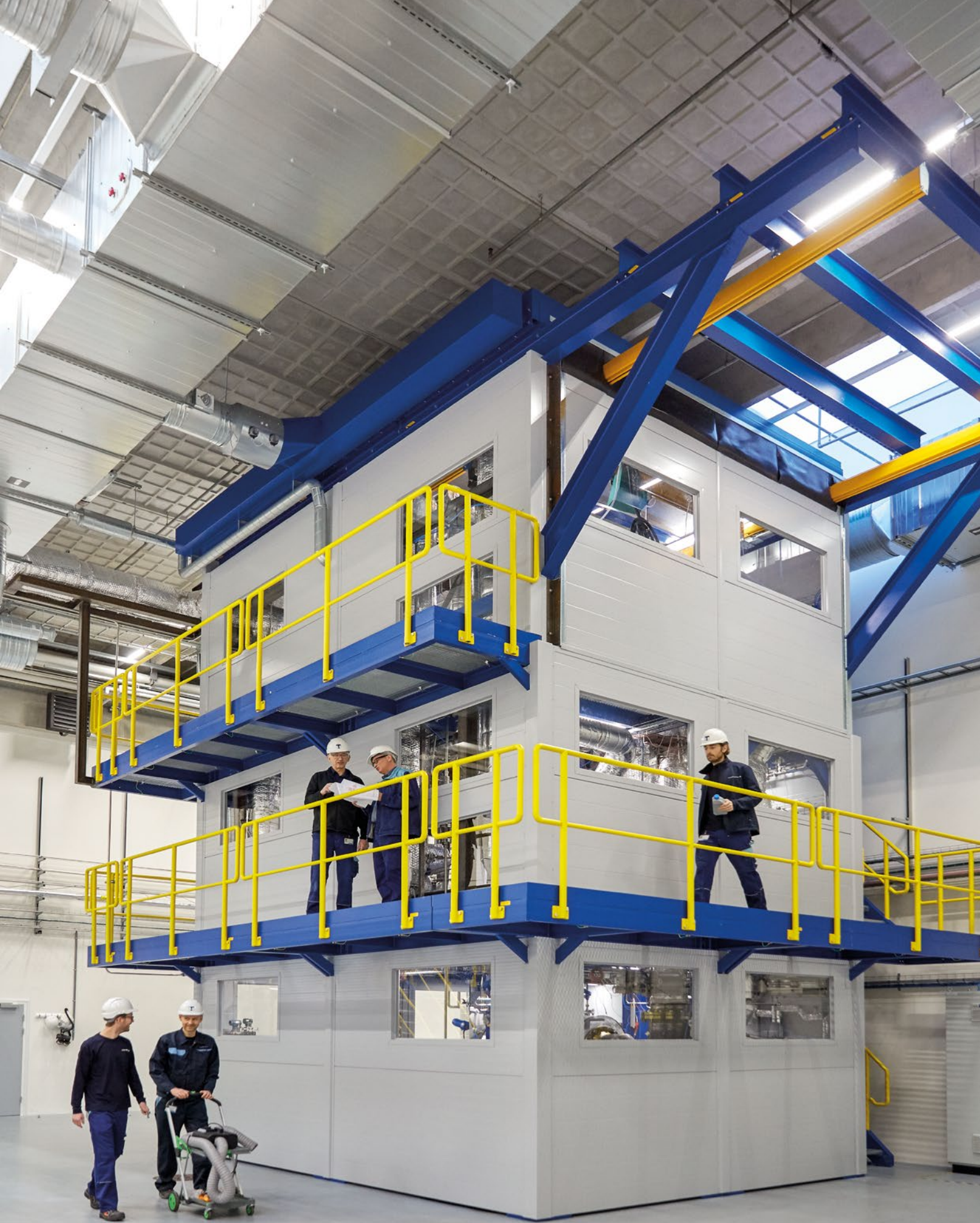
Braskem and Topsoe have entered a partnership to build and operate a demonstration plant that uses sugar as feedstock to produce more than 100 tons per year of glycolaldehyde, which is the precursor for MEG that is used to produce bio-based PET plastic.
